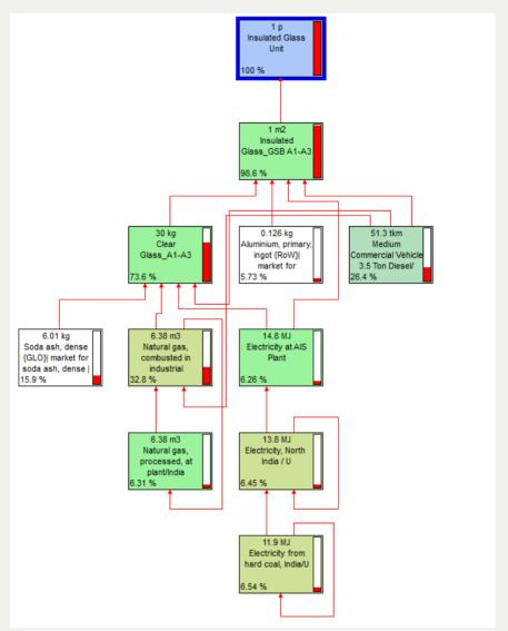
Figure: - Network diagram for GWP-GHG results as kg CO2 eq. for 1m2 of Insulated Glass Unit
