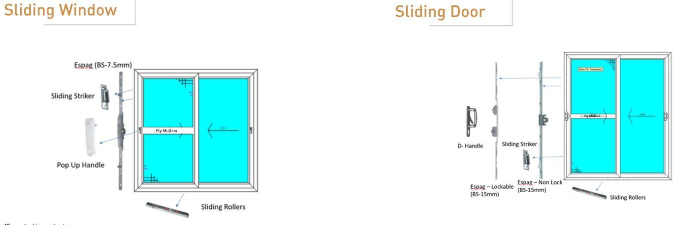
\*Espag: Locking mechanism \*\*3D Hinges: Facilitates movement of door panels
