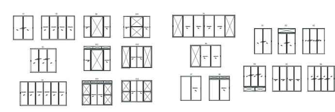
Available Combination in Slider Doors & Windows- 2T2P, 2T3P, 2T4P, 3T3P, 3T6P, 3T2P+1M, etc. (T-Track, P-Panel, M-Mesh Panel)
