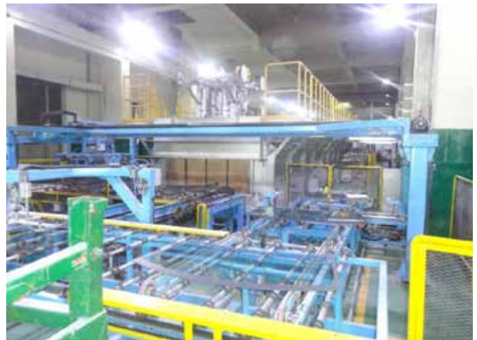
Bending Furnace for car glass
