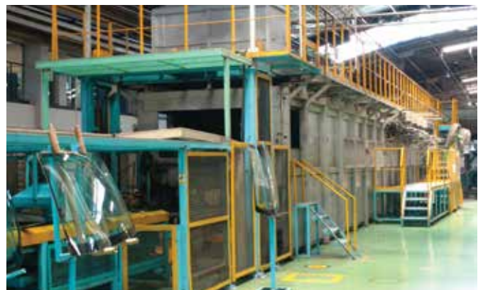
Laminated Bending Furnace
