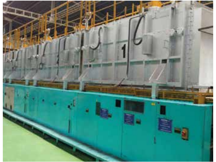
Tempering Furnace for Sidelites
