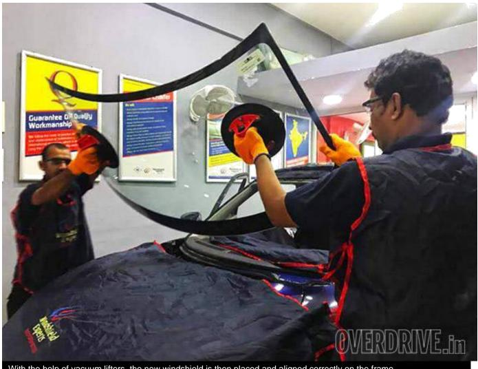
With the help of vacuum lifters, the new windshield is then placed and aligned correctly on the frame
