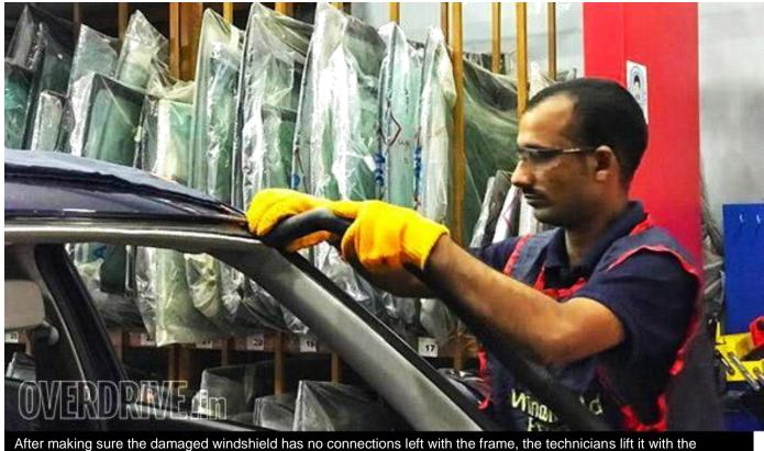
After making sure the damaged windshield has no connections left with the frame, the technicians lift it with the help of two vacuum based lifters. The remains of the old adhesive on the frame is peeled off
