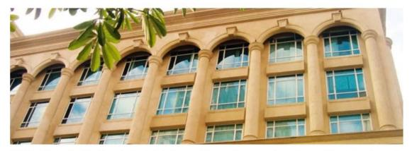
AIS Tinted Heat-absorbing Glass is a body tinted glass which absorbs energy from solar radiation. It, therefore, cuts down the sun's heat, enabling greater convenience and comfort inside the building, while enhancing the aesthetic appeal of the building from outside.
