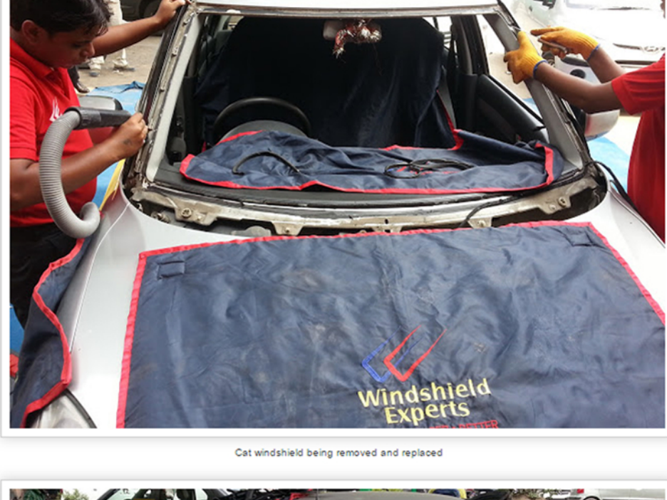
Cat windshield being removed and replaced
