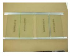
Fig 9 Silicone butt-joined samples used for Florida edge stability study
