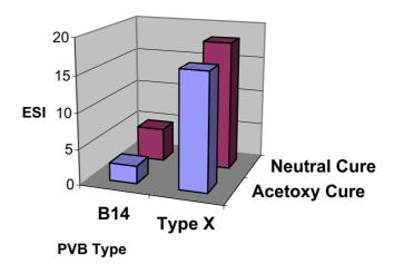
Weathering of SGP Laminates with Silicone Sealants
