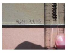
SGP laminate exposed edge after 61 months of Florida exposure - no edge defects
