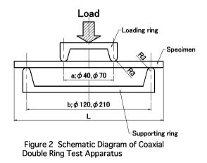
of strength distribution, and the allowable mechanical strength is decided for each glass thickness. Fig.2 shows the testing apparatus.
