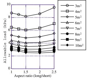
Figure 5 Allowable load (thickness 19mm)
