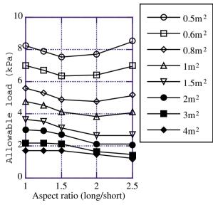
Figure 4 Allowable load (thickness 6mm)
