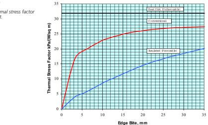
massive heat sink with minimal thermal isolation. Such a situation occurs if the edge bite is encased in concrete or in a thick-walled metal frame. This case represents the most critical situation for the development of thermal stresses. In addition, the magnitude of thermal stress estimated using this assumption is believed to provide a conservative estimate of the maximum tensile stress that can be generated in a glass plate subjected to a linear shadow pattern.
