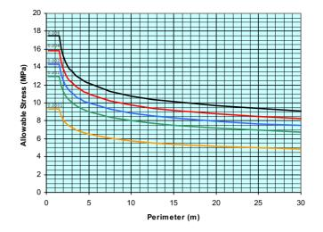
magnitude of the thermally induced stresses and an edge strength failure prediction model (ESFPM) that is used develop the method for determining the significance of the calculated thermal stress in monolithic annealed glass.
