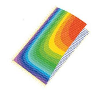
The mechanical properties like shear modulus of the pvb interlayer influence the performance of the laminated glass. The new high performance interlayer from DuPont called Sentry Glass® Plus is an example of the improved benefits from using modified interlayers.
