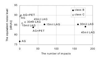
Figure 2 Relationship between the number of impacts and the equivalent noise level
