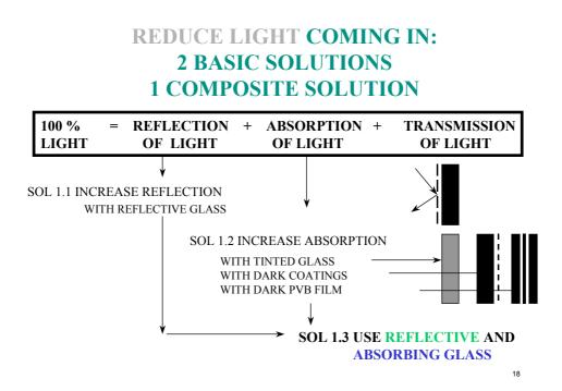
To improve internal comfort levels and decrease air conditioning costs it is important to reduce the IR energy entering. This can be done in 3 basic plus 2 composite ways:
