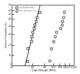
Figure 6. Weibull distributions of strength data for Sandbelt edge before and after heat strengthening
