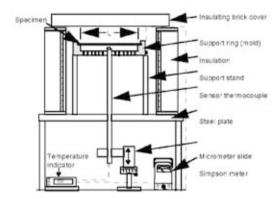
Figure 10. Beam bending viscometer
