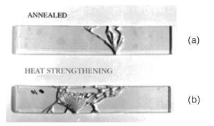
Figure 9. (a) Fracture pattern for Twin Cut edge before heat strengthening; (b) fracture pattern for Twin Cut edge after heat strengthening
