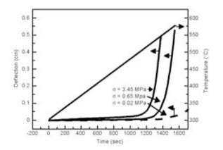
Figure 11. Deformation of glass specimen as function of stress, temperature and time
