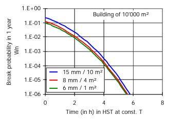
Figure 3: Calculated break probability for HS-processed glass panes on a building with 10000 m<sup>2</sup> of glass surface, as a function of the residence in HST time at a constant temperature of 290°C. After 2 hours of holding time, the probability is next to 0.01. This means that very probably no break will happen. The glass is safe.
