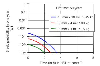
Figure 2: Calculated one year's breaking probability for HS-Processed glass panes of different
