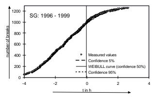
Figure 2: WEIBULL evaluation of 1258 breaks recorded in one type of HST furnace. Mean heating time was 6 h. When reaching constant temperature, 1012 breaks, i.e. 80.4% of the total number, have already happened.
