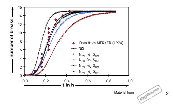
Figure 1: Our new kinetic results fit MERKER's laboratory results obtained from NiS inclusions he located in drawn glass sheets.
