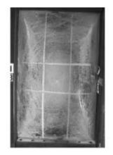
Fig 3 Post test photograph of ionoplast laminate.
