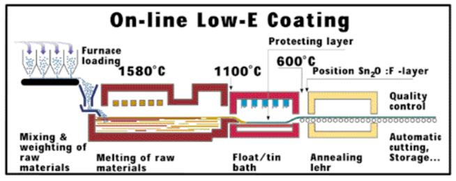
Figure 1: The float and the coating line
