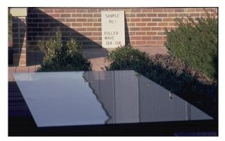
Figure 4 **R**oller Wave Distortion – Reflected Image RW Factor = 66.00 mdpt (approx.) Photo Courtesy of S.W. Joehlin, Inc.
