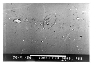
Figure 7 Tempred Glass with Bottom Surface Markin @ 50x Microscopic Paint Debris
