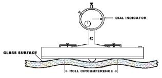
Figure 1 Flat Bottom Gauge For Measuring Roll Wave
