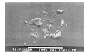
Figure 8 Tempered Glass with Bottom Surface Marking @ 500x Microscopic Glass Dust
