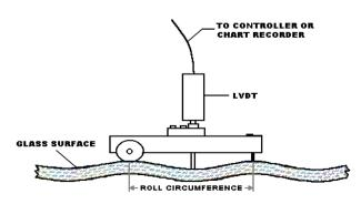
Figure 2 Three Point Gauge For Measuring Roll Wave
