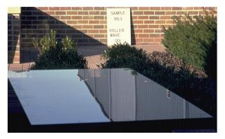
Figure 3 Roller Wave Distortion – Reflected Image RW Factor = 13.00 mdpt (approx.) Photo Courtesy of S.W. Joehlin, Inc.
