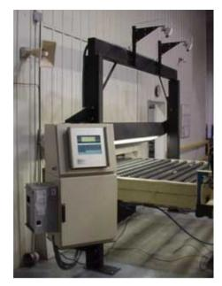
Figure 4: LiteSentry™ Roll Distortion Measurement System
