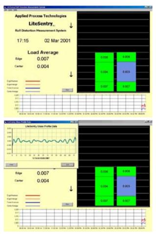
Figure 6a & 6b: Operator Display without and with sheet profile
