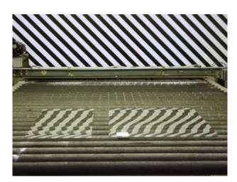
Figure 1: A View of Glass Sheets in Front of a Zebra Board
