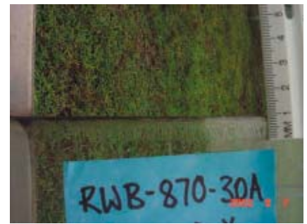
Fig 6 Open edge of a Type X laminate after 54 months of Florida exposure
