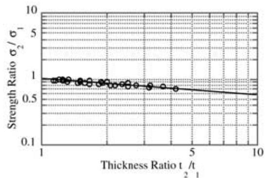
Figure 3 The Relationship between Thickness Ratio and Strength Ratio
