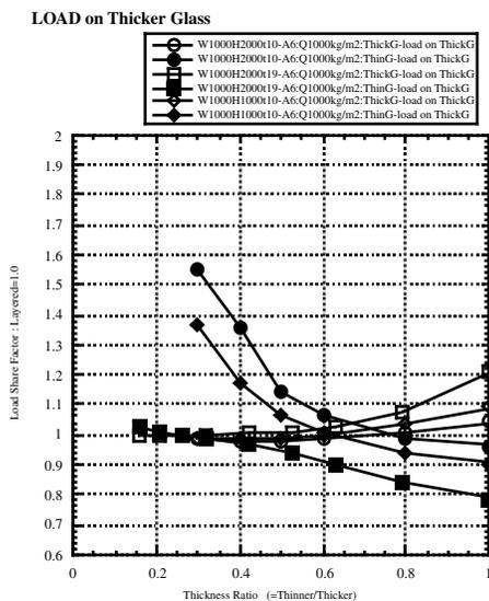
Figure 6 The Relationship between Thickness Ratio and Load Share Factor
