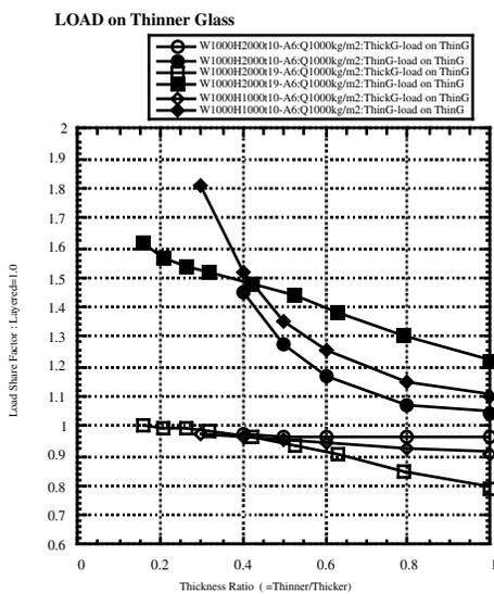
Figure 7 The Relationship between Thickness Ratio and Load Share Factor
