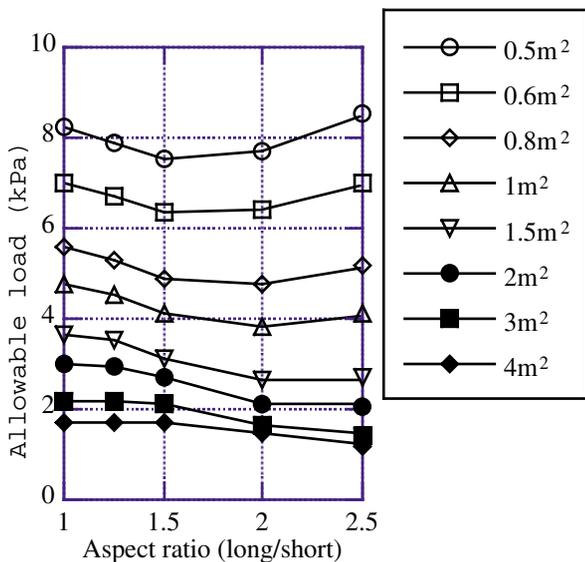
Figure 4 Allowable load (thickness 6mm)
