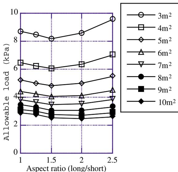
Figure 5 Allowable load (thickness 19mm)
