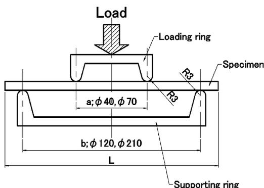
Figure 2 Schematic Diagram of Coaxial Double Ring Test Apparatus
