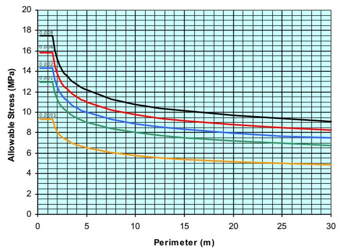
magnitude of the thermally induced stresses and an edge strength failure prediction model (ESFPM) that is used to develop the method for determining the significance of the calculated thermal stress in monolithic annealed glass.
