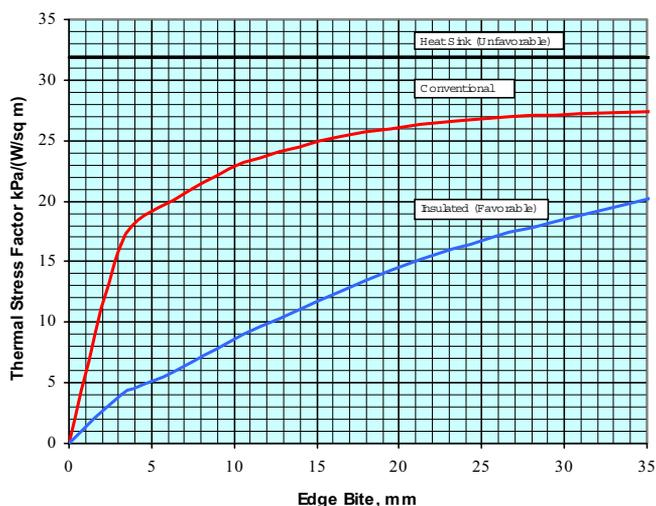
massive heat sink with minimal thermal isolation. Such a situation occurs if the edge bite is encased in concrete or in a thick-walled metal frame. This case represents the most critical situation for the development of thermal stresses. In addition, the magnitude of thermal stress estimated using this assumption is believed to provide a conservative estimate of the maximum tensile stress that can be generated in a glass plate subjected to a linear shadow pattern.
