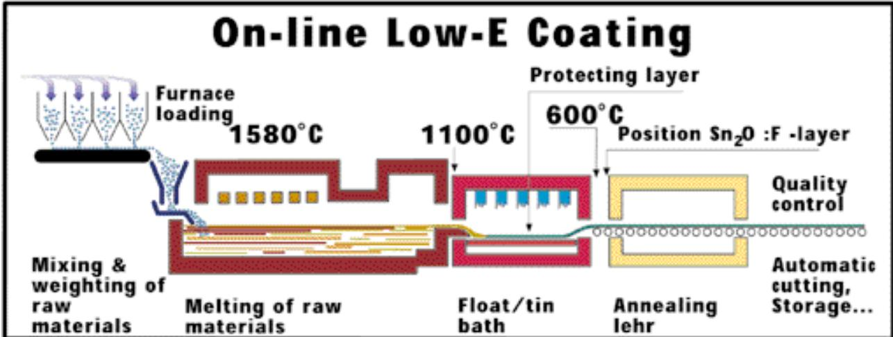
Figure 1: The float and the coating line
