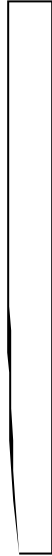
Figure 3. Section through heavy glass showing an exaggerated thickness change near one edge of the float ribbon. (Not to scale).
