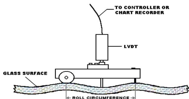
Figure 2 Three Point Gauge For Measuring Roll Wave
