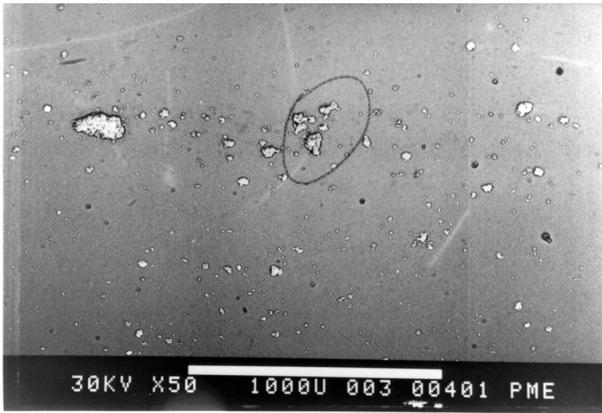
Figure 7 Tempered Glass with Bottom Surface Markin @ 50x Microscopic Paint Debris
