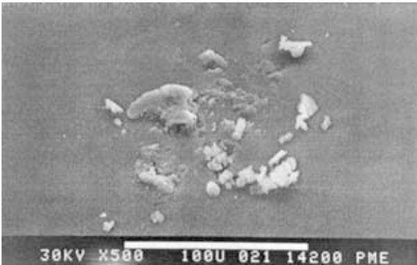
Figure 8 Tempered Glass with Bottom Surface Marking @ 500x Microscopic Glass Dust
