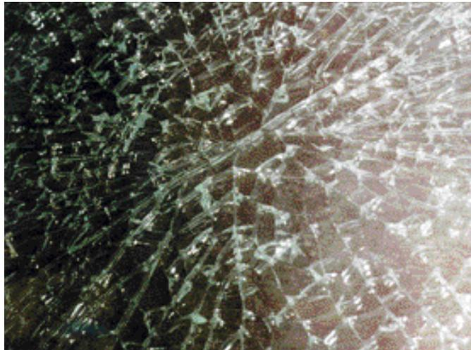
since 1965, much of the glass it has toughened to the routine use of the online heat soak process. The company's claimed conversion rate is presumably derived from repeated heat soak testing on the same panes of toughened glass.
