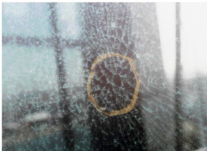
Where a nickel sulphide inclusion of critical size (NSICS) occurs in the inner portion of toughened glass, which is already in tension, the resulting increased tensile stress can exceed the strength of the glass.
