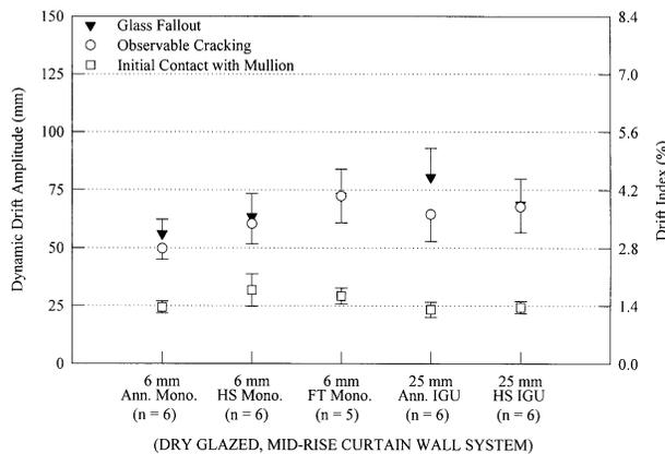
Figure 4. Effects of glass surface prestress
