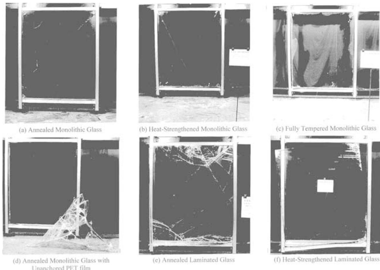
Figure 3. Typical failure patterns in various architectural glass types after in-plane dynamic racking tests
