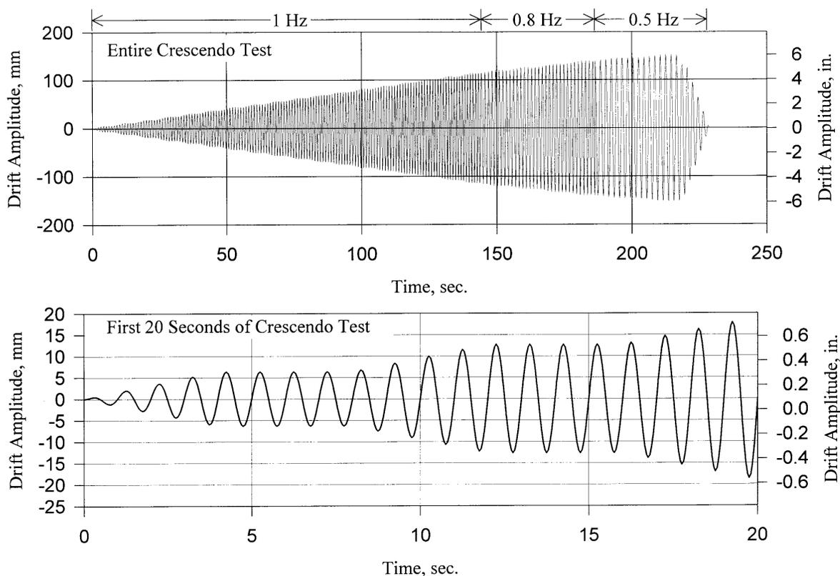
Figure 2. Drift time history in the crescendo test used for mid-rise architectural glass specimens
