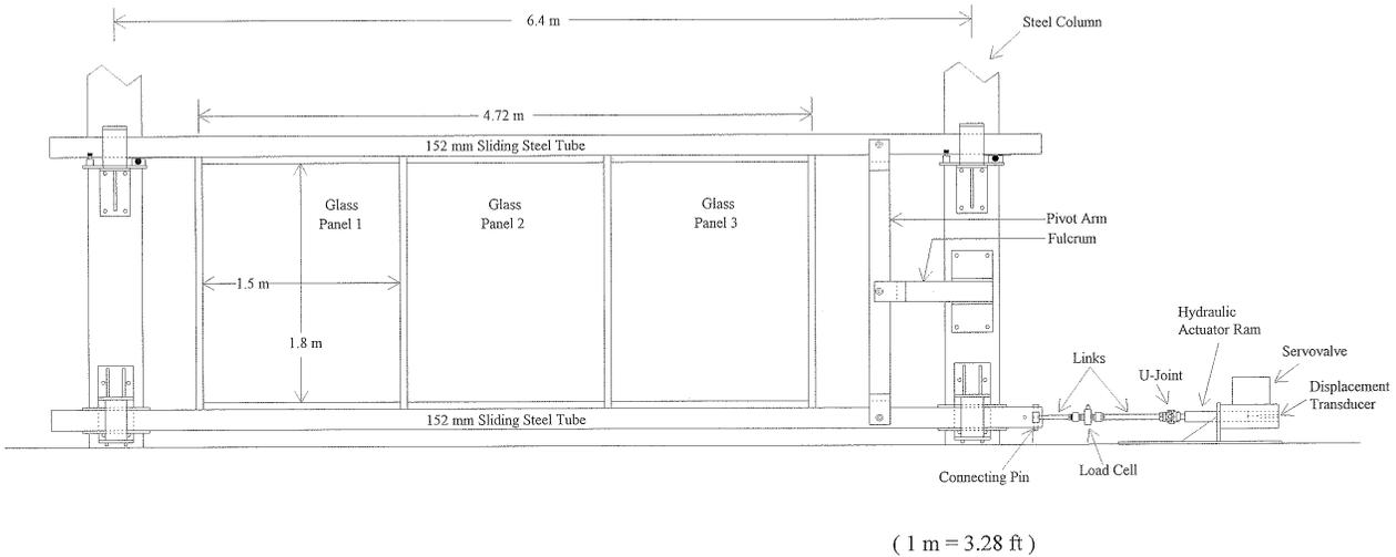
Figure 1. Dynamic racking test facility
