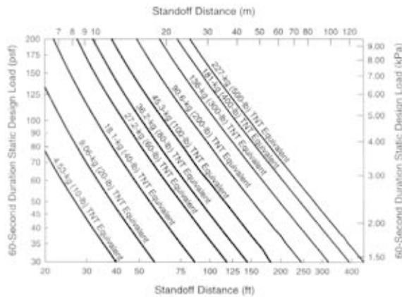
Figure 2. Relationship Between TNT Charge Size, Standoff Distance, and Design Load.
