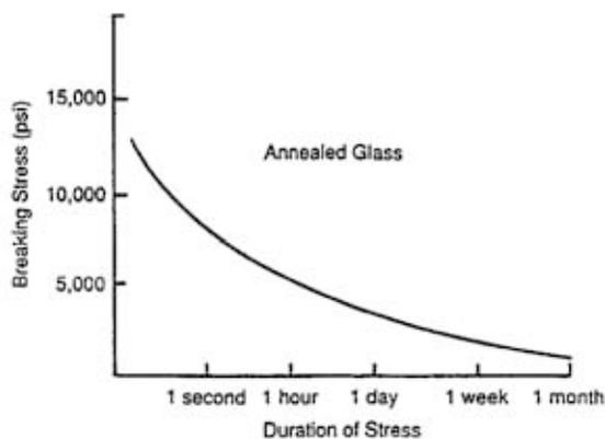
Figure 1. Breaking Stress versus Stress Duration for Annealed Window Glass.
