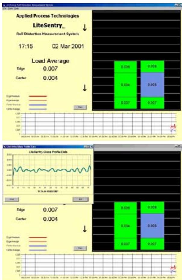
Figure 6a & 6b: Operator Display without and with sheet profile
