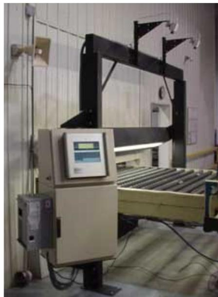
Figure 4: LiteSentry™ Roll Distortion Measurement System
