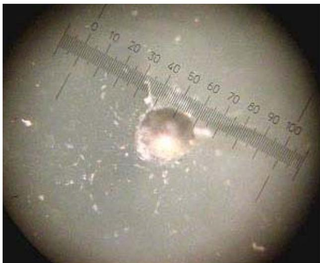
is very impure then the heat soaking process will not cause failure in the oven. However, this impure stone can cause failure in the installed panel at a later date. This is because of other factors such as membrane, bending or thermal stresses and crack growth acting on the vent associated with the inclusion. An example of a fracture origin from such a case is illustrated in figure 2.
