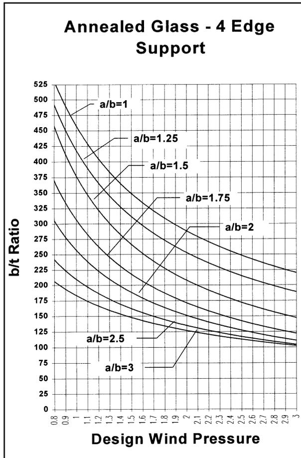
Figure 4. New Design Chart - Ultimate Limit State Loading.
