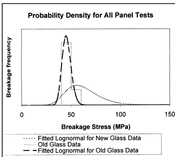
Figure 3. Breakage Data for 30 Year Old Glass.
