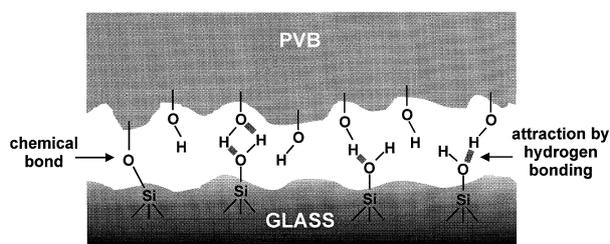
Figure 5. PVB-glass bonding mechanism.
