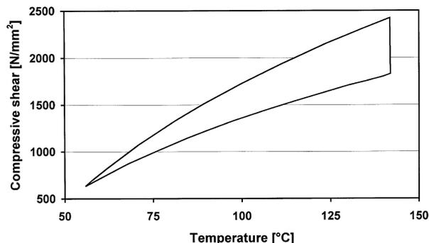
Figure 6. Compressive shear adhesion versus autoclave temperature.
