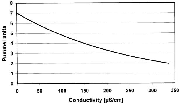
Figure 7. Pummel adhesion against conductivity of rinsing water.
