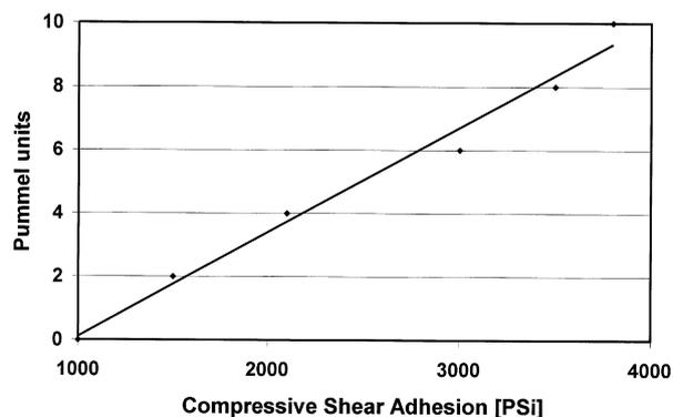
Figure 3. Correlation between Pummel and Compressive shear test.
