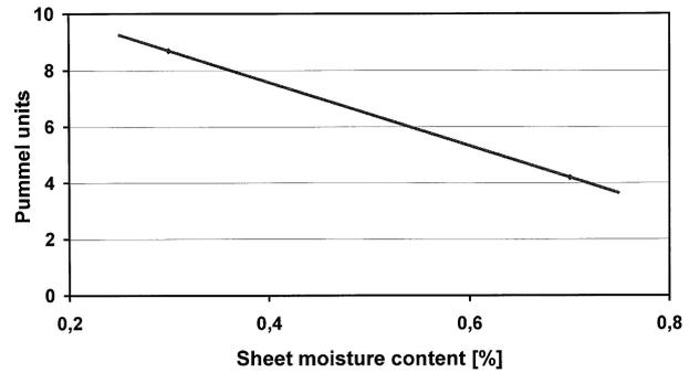
Figure 9. Pummel adhesion versus sheet moisture content.
