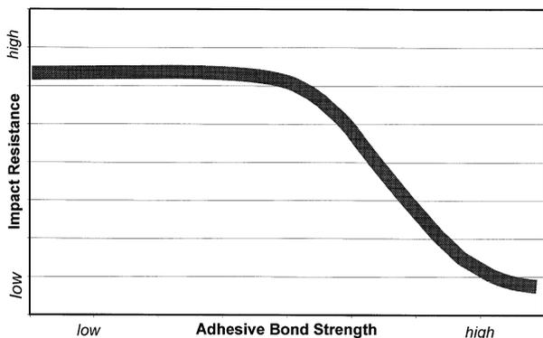
Figure 1. Impact resistance as a function of adhesive bond strength.
