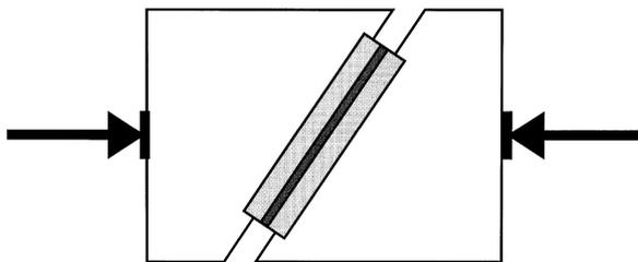
Figure 2. Position of the test specimen in the compressive shear test.
