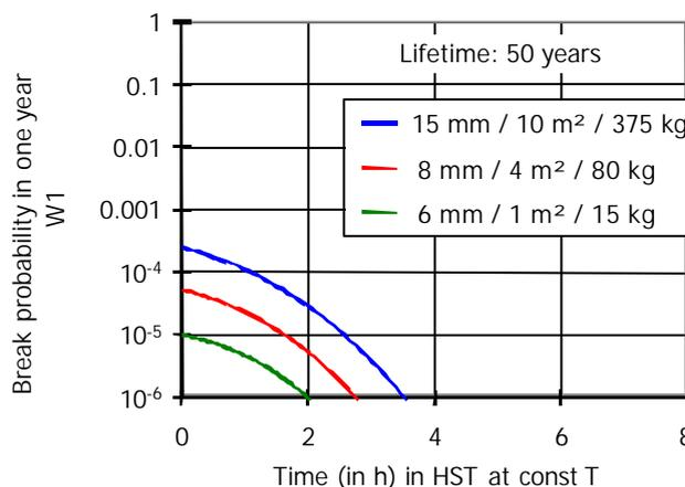
Figure 2: Calculated one year's breaking probability for HS-Processed glass panes of different
