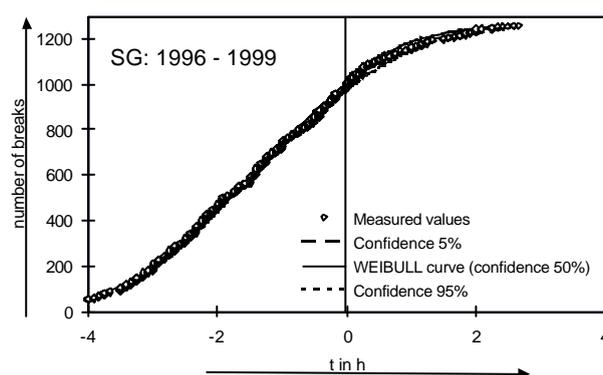
Figure 2: WEIBULL evaluation of 1258 breaks recorded in one type of HST furnace. Mean heating time was 6 h. When reaching constant temperature, 1012 breaks, i.e. 80.4% of the total number, have already happened.
