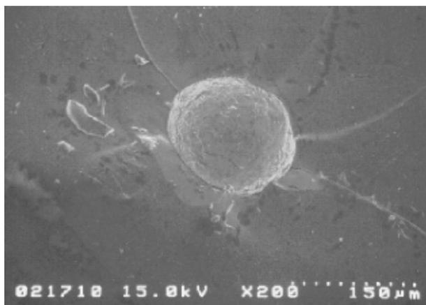
Figure 1. NiS particle after spontaneous failure of tempered glass.
