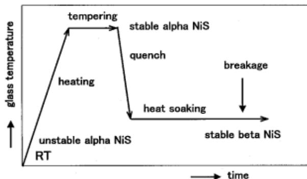
Figure 5. Schematic diagrams of new heat soak treatment.
