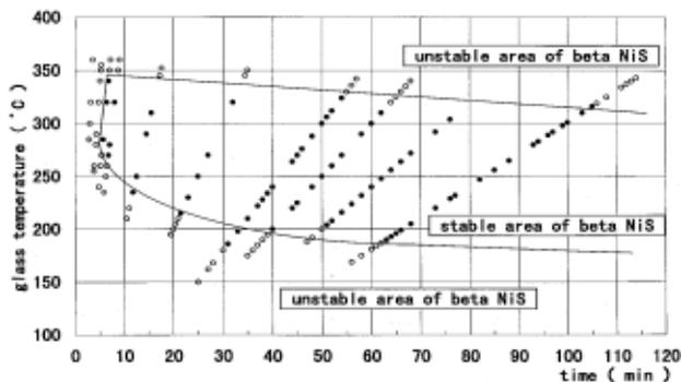
Figure 4. T-T-T diagram of NiS at the different rate of rising temperature.
