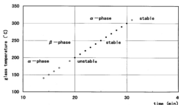
Figure 3. Time-temperature-transformation (T-T-T) diagram of crystalline NiS.
