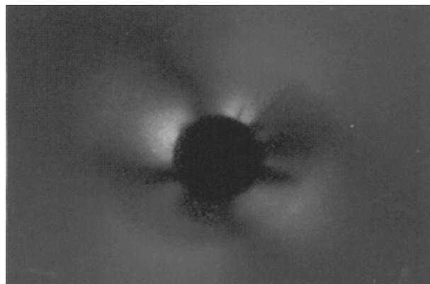
Figure 2. Perfectly transformed beta phase of NiS in the glass after heat soak treatment.
