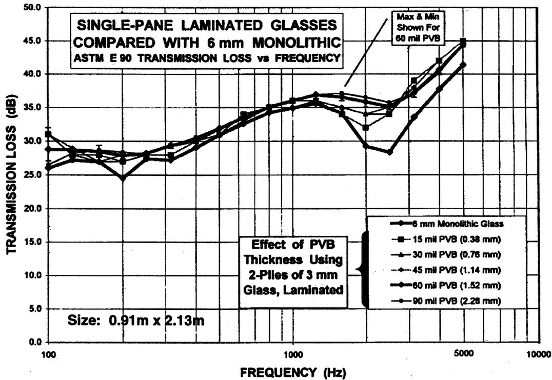
Figure 8. Effect of Lamination on 6 mm Transmission Loss.
