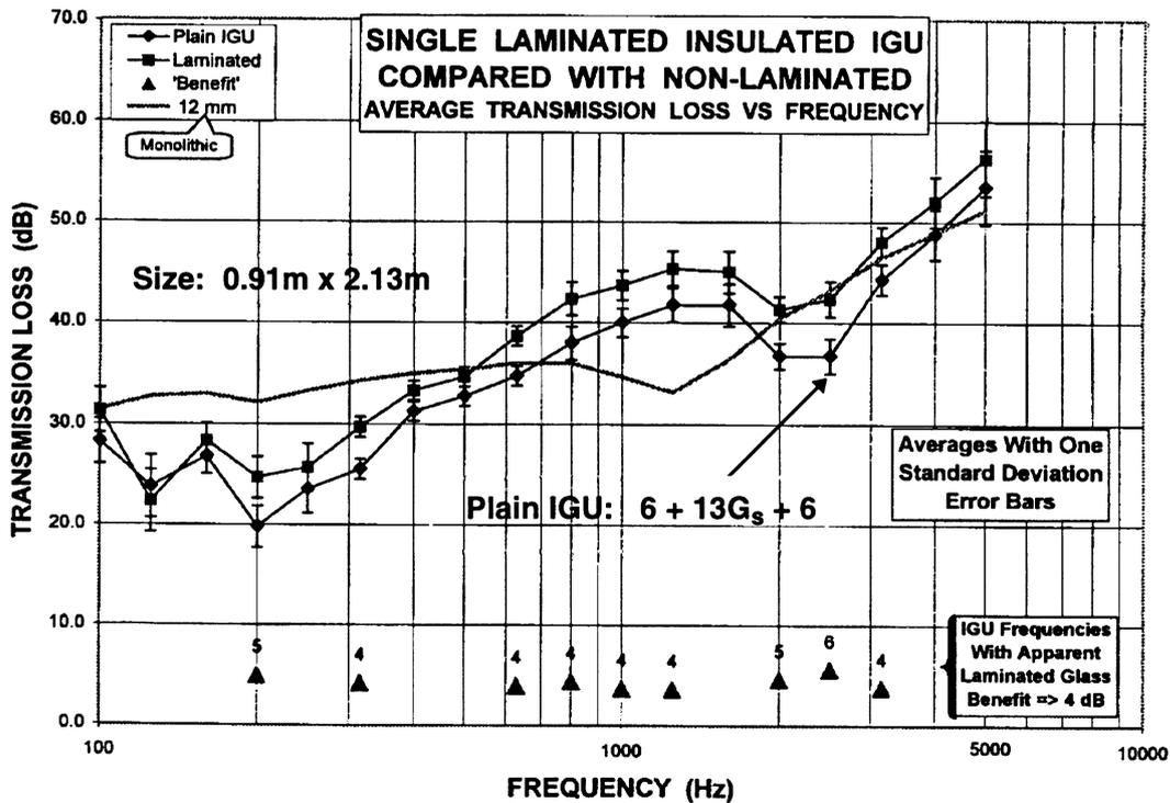
Figure 9. Effect of Lamination on 12 mm Insulated Glazing.
