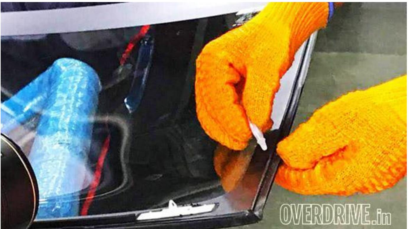
A fresh coat of new adhesive is applied on the edges of the new windshield
