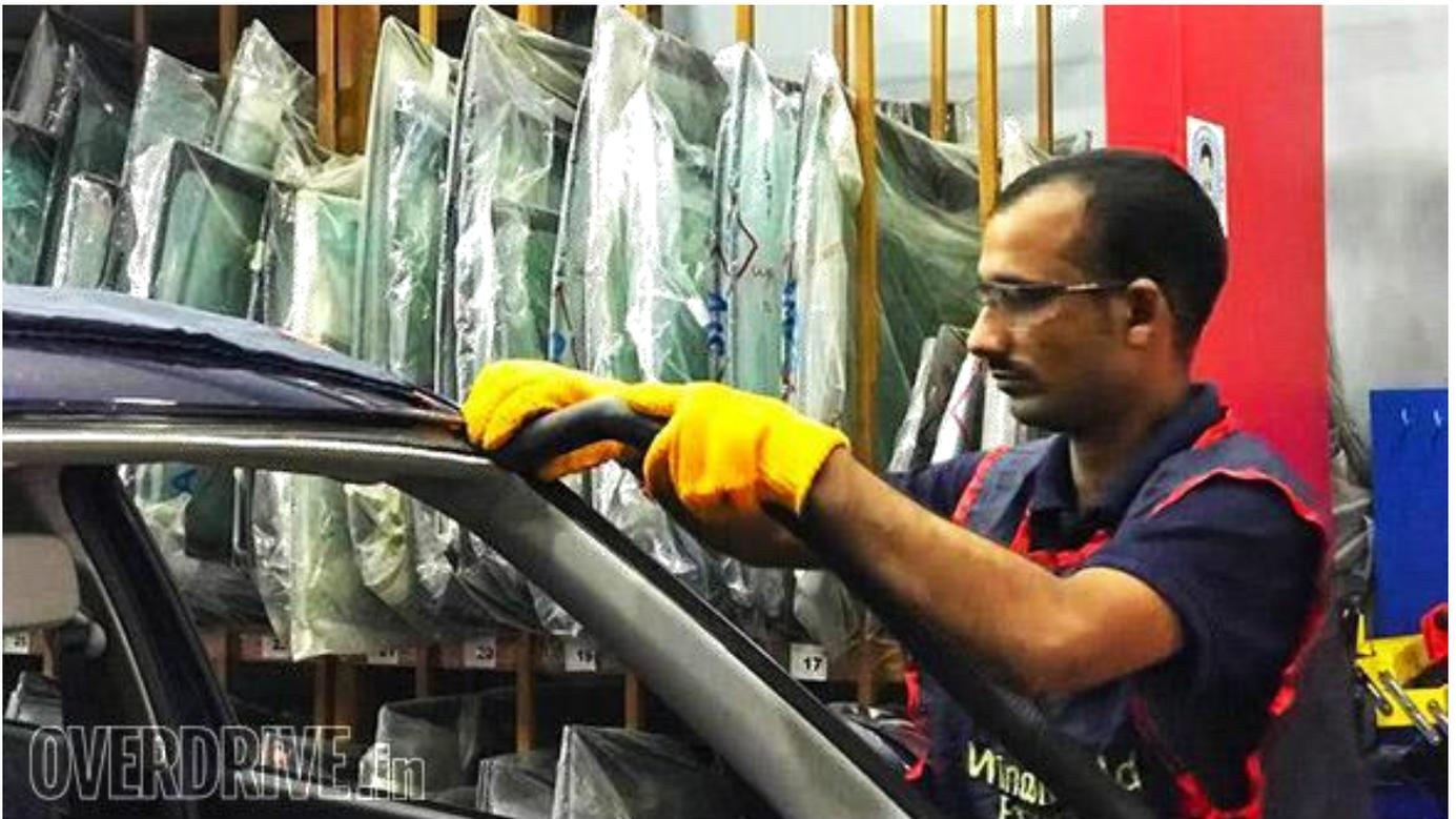
After making sure the damaged windshield has no connections left with the frame, the technicians lift it with the help of two vacuum based lifters. The remains of the old adhesive on the frame is peeled off
